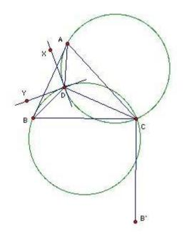
Take B' so that CB = CB',  $\angle BCB' = 90^{\circ}$  and B' is on the opposite side of BC to A. It is easy to check that ADB, ACB' are similar and DAC, BAB' are similar. Hence AB/BD = AB'/B'C and CD/AC = BB'/AB'. It follows that the ratio given is BB'/B'C which is  $\sqrt{2}$ .
